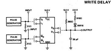
"1" set-up time. tsi "0" set-up time. tso "1" hold time. thj "0" hold time. tho Pulse width
