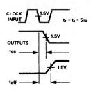
Transfer rate & min clock "1" level: check that binary outputs are changing.
