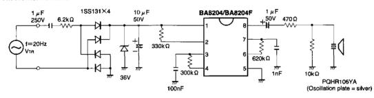
Fig. 4 Ringer threshold voltage measurement circuit
