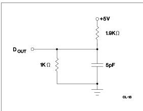
Figure 1. Output Load A
