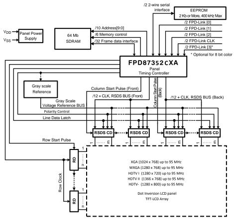
Figure 1. Block Diagram of the LCD Module
