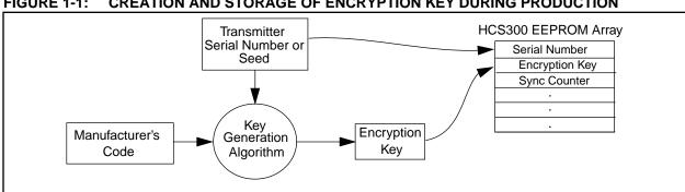
FIGURE 1-1: CREATION AND STORAGE OF ENCRYPTION KEY DURING PRODUCTION
