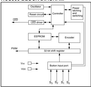
The HCS300 combines a 32-bit hopping code generated by a non-linear encryption algorithm, with a 28-bit serial number and six status bits to create a 66-bit transmission stream. The length of the transmission eliminates the threat of code scanning and the code hopping mechanism makes each transmission unique, thus rendering code capture and resend (code grabbing) schemes useless.
