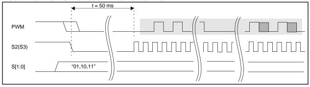
FIGURE 4-4: TRANSMISSION WORD FORMAT DURING SYNCHRONOUS TRANSMISSION MODE
