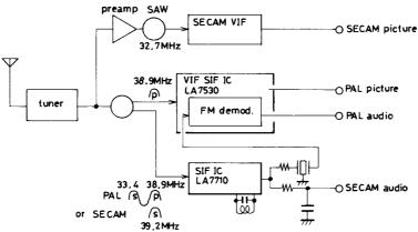
(Note) \*1 When selecting the PAL/SECAM, the LLD tuning point of the LA7710 must be changed over (38.9MHz  $\rightarrow$  39.2MHz).
