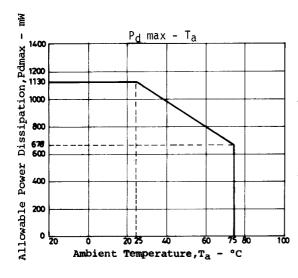
The loss of the following waveform is allowed at Ta=60°C
