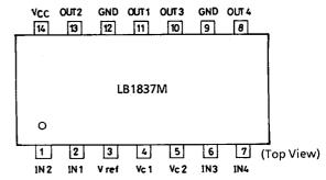
Note: Both GND pins must be grounded.
