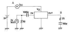
Fig. A Propagation Time, Transient Time
