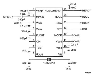
Caution: If the RST pin is unused, it must be connected to ground.
