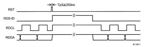
Caution: After an RST input, the RDCL and RDDA outputs stop at the high level until the first RDS ID detection.
