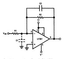
Parasitic input capacitance C1  $\simeq$  (3 pF for LF351 plus any additional layout capacitance) interacts with feedback elements and creates undesirable high frequency pole. To compensate, add C2 such that: R2C2  $\simeq$  R1C1.
