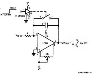
\*Low leakage capacitor • 50k pot used for less sensitive V<sub>OS</sub> adjust LF351
