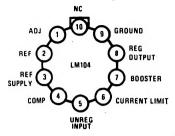
Note: Pin 5 connected to case.
