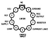
Note: Pin 5 connected to case.
