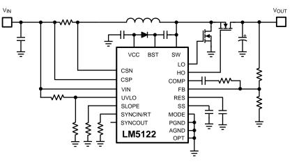
Figure 1. SIMPLIFIED APPLICATION DIAGRAM
