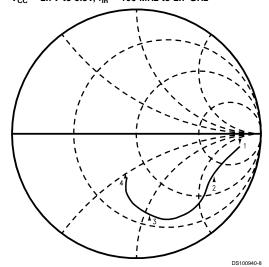
Marker 1 = 100 MHz, Real = 364,  $I_{mag}$  = -253 Marker 2 = 1 GHz, Real = 104,  $I_{mag}$  = -136 Marker 3 = 2 GHz, Real = 26,  $I_{mag}$  = -53 Marker 4 = 2.7 GHz, Real = 36,  $I_{mag}$  = -23
