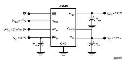
FIGURE 7. SSTL-2 Implementation with higher voltage rails
