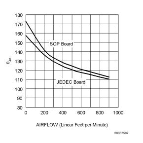
FIGURE 2.  $\theta_{JA}$  vs Airflow (SO-8)
