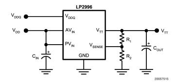
FIGURE 10. Increasing VTT by Level Shifting
