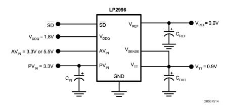
FIGURE 9. DDR-II Termination with higher voltage rails
