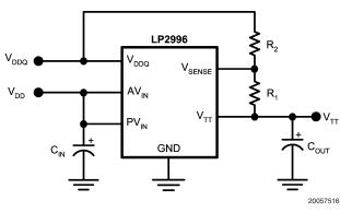
FIGURE 11. Decreasing VTT by Level Shifting
