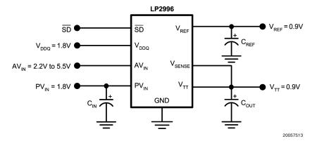
FIGURE 8. Recommended DDR-II Termination
