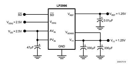
FIGURE 14. Typical SSTL-2 Application Circuit for Motherboards
