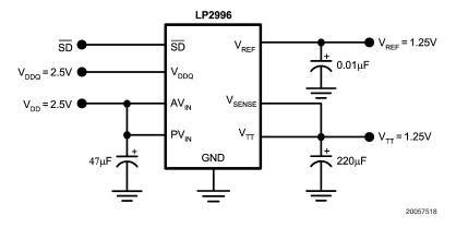
FIGURE 13. Typical SSTL-2 Application Circuit
