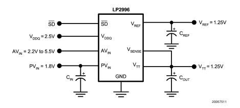
FIGURE 6. Lower Power Dissipation SSTL-2 Implementation
