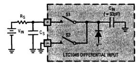
Figure 1. Equivalent Input Circuit
