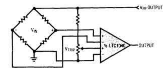
Figure 6. Ratiometric Network Driven by VPP
