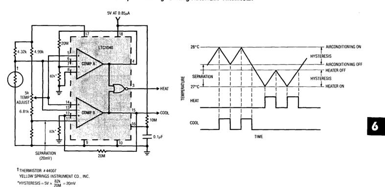
Complete Heating/Cooling Automatic Thermostat
