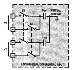
Figure 2. Dual Differential Equivalent Input Circuit
