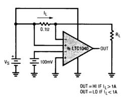
Figure 4. Load Current Detector
