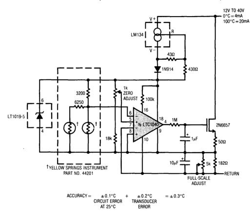
2-Wire 0°C to 100°C Temperature Transducer with 4mA to 20mA Output
