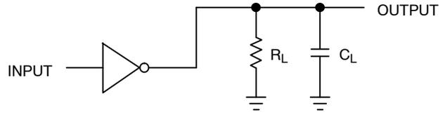
A 1-MHz square input wave is recommended for propagation delay tests.
