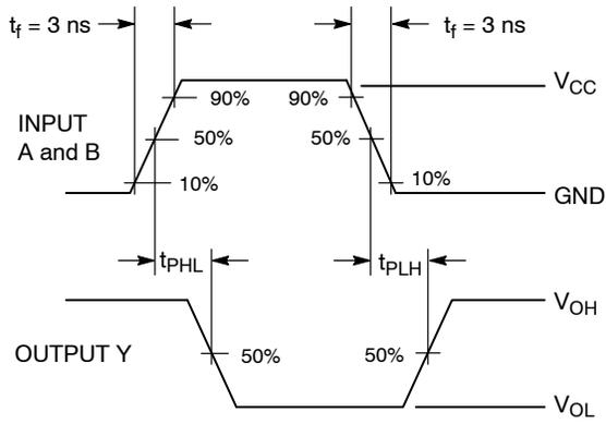
Figure 3. Switching Waveform
