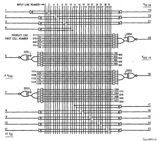
JEDEC logic array cell number = product line first cell number + input line number
