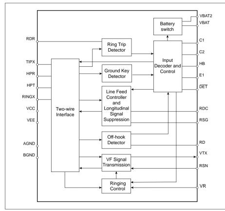
Figure 1. Block diagram.
