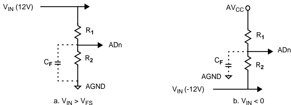
Figure 61. Measurement of Positive and Negative Voltages
