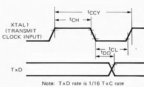
**Figure 4a. "Transmit" Timing with External Clock**
