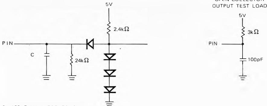
$C = 130pF \text{ MAX. FOR } DB_0\text{-}DB_7$
