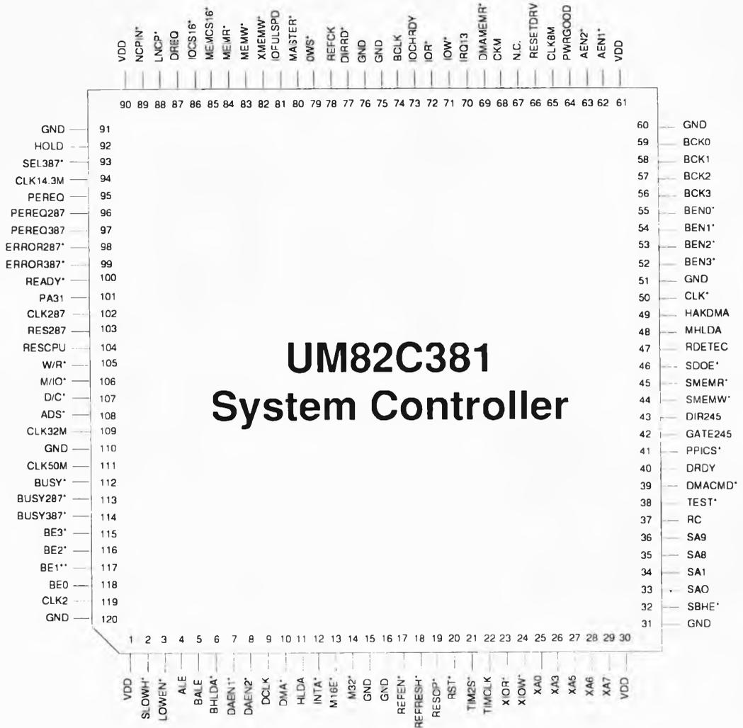
Figure 2. Pin Configuration
