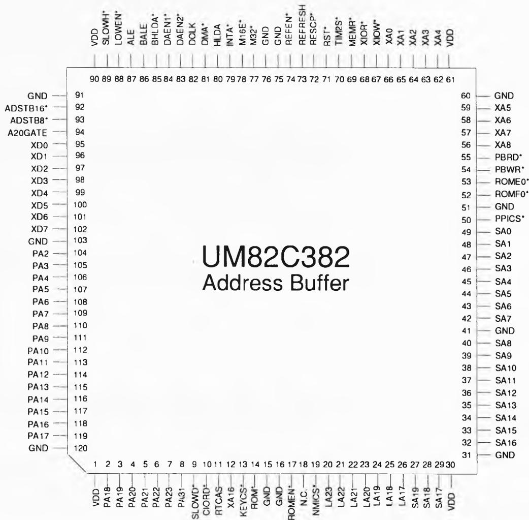
**Figure 2. Pin Configuration**
