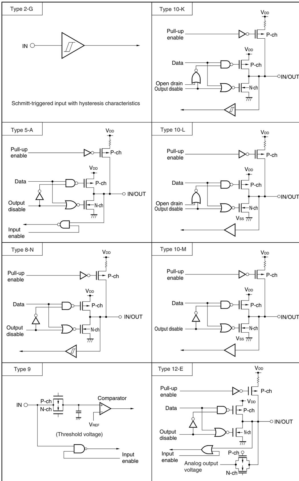
Figure 4-1. Pin I/O Circuits (2/2)
