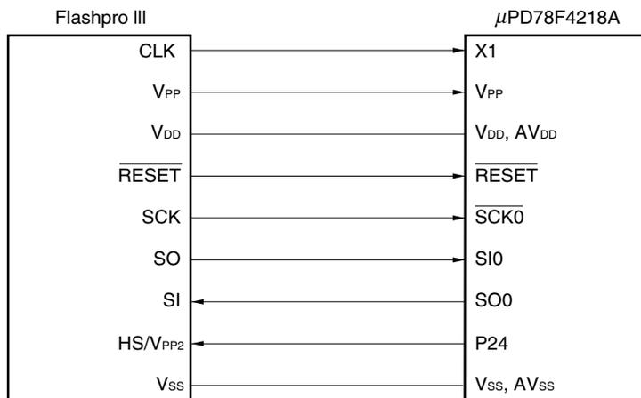
**Figure 6-4. Connection of Flashpro III in UART Mode (When Using UART)**
