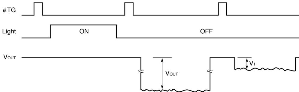
$$\text{IL (\%)} = \frac{V_1}{V_{\text{OUT}}} \times 100$$
