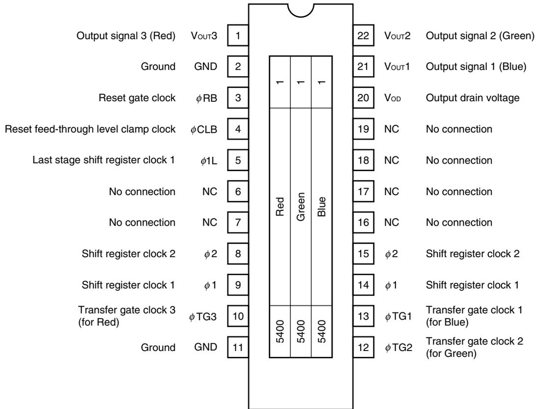
**Caution** Connect the No connection pins (NC) to GND.
