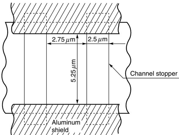
**PHOTOCELL ARRAY STRUCTURE DIAGRAM (Line spacing)**
