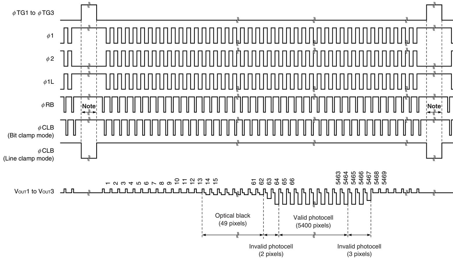
**Note** Set the  $\phi$ RB and  $\phi$ CLB (Bit clamp mode) to high level during this period.
